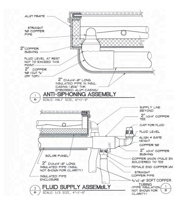
The "Anti-Siphoning Assembly" consists of brazed fittings configured so that the reduction in pipe size is done in the vertical rather than horizontal plain. This prevents any possibility for thermal siphoning.
