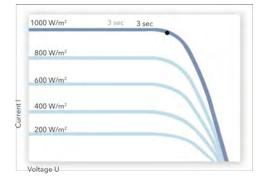
Typical Current-Voltage-curve of a photovoltaic panel. By employing MPP tracking every three seconds, the D5 pumps always automatically achieve maximum performance at any given insolation.
