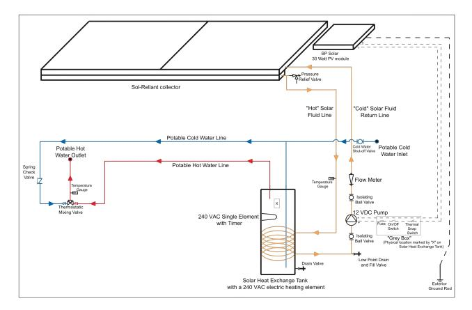
**STEP 3:** Place a Tee in the line downstream of the shut off valve. From one of the two open ports of the Tee, plumb to the cold inlet port on the top of the solar tank. The remaining open port of the cold water tee needs to be plumbed to the cold side of the tempering valve (marked "Cold").
